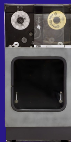
1951: The Uniservo 1 served as an input-output device to replace punched cards on the new Univac 1 computer.
