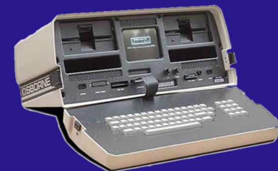
1981: The Osborne 1 is the first commercially successful portable microcomputer, released by Osborne Computer Corporation. It weighs 10.7 kg, costs US$1,795.
